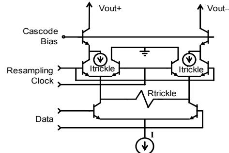
Fig. 2 DAC current switch
