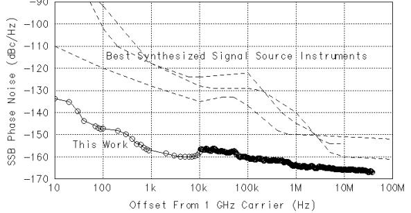
Fig. 7 Phase noise at 1 GHz of this DAC at 7.2 GSa/s and of synthesized signal generator instruments
