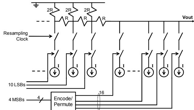
Fig. 1 DAC Core simplified schematic
