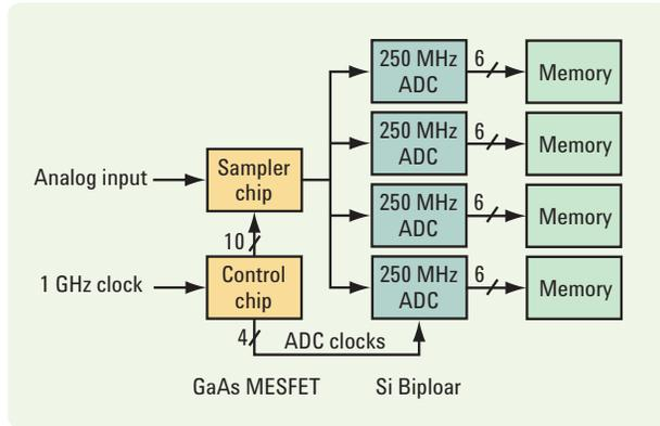
Figure 8. Complete block diagram of 1 GS/s ADC system.
