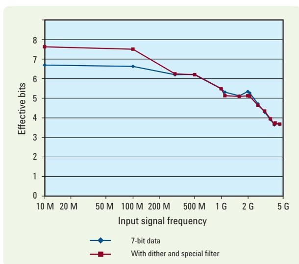
**Figure 11. Accuracy of the 8 GS/s ADC.**
