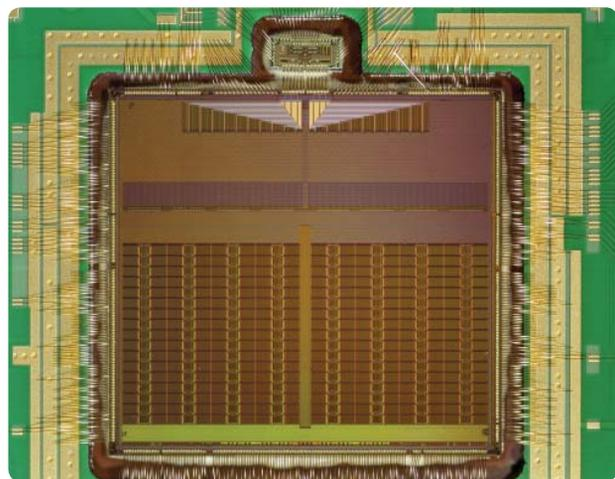
**Figure 12. 20-GS/s CMOS ADC chip**
