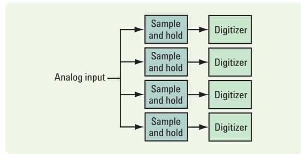
**Figure 5. Four 250 MS/s sample and hold circuits and ADCs are time-interleaved to produce a 1 GS/s system.**
