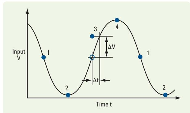
**Figure 6. A small sample and hold timing error can produce a significant error in the sampled voltage.**
